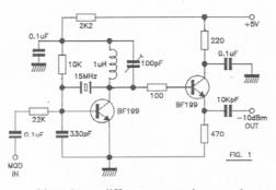
At this point a different approach was taken: modify a FM modulated cristal oscillator (VXO) in a way to make it operating with a SAW. A"standard " building block was used (Fig. 1),a proven oscillator used in our projets for 15 years. This circuit is capable of FM modulating a 15 Mhz fundamental cut quarz cristal at +/- 4Khz,
