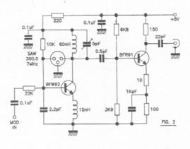
The current draw from a 5 V supply is tipically 25 mA; the supply should be stabilised, otherwise change in tuning and in modulation will occur.
