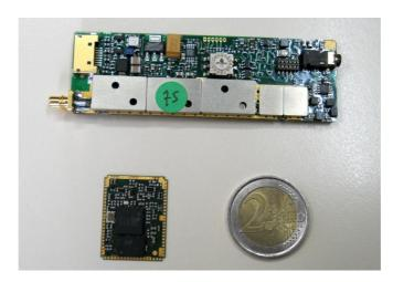
In this image we can see the dimentional comparison with a class 1 BT board and the equivalent LPD technology at 433.92 MHz. Dimensions are ¼ and the cost... too!
